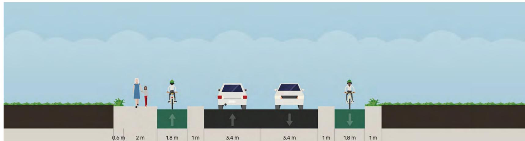
Figure 27. Queen Street indicative cross section design
